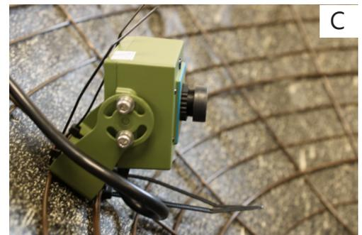
**Step 4:** Before flipping, make sure to tighten the bracket with the Allen key, and position the camera so its facing the entrance. Please refer to image "C". You can then cut off the tails of the cable ties if you want a cleaner look.
