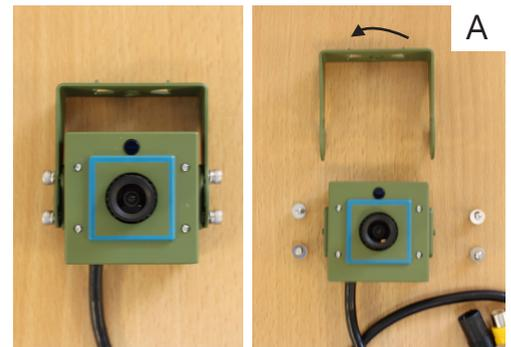
**Step 2:** To get an idea of the placement of the camera. We generally recommend placing the camera opposite the entrance on the rear of the house. This will give you a clear view of the entrance. To make sure the camera is the correct way up make sure the small lens is on top of the large lens. You when you flip the house when finished it will then appear below the lens. Refer to image "A" for now.
