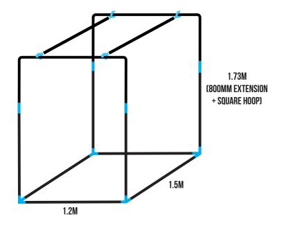
**PLEASE NOTE:** A mallet is usually required to tap the joiners into the tubes. Please ensure the joiners are fully submerged into the aluminium.
