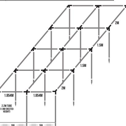
**PLEASE NOTE:** A mallet is usually required to tap the joiners into the tubes. Please ensure the joiners are fully submerged into the aluminium.
